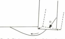
Fig. 8. Displacement of wall base due to bearing capacity failure
