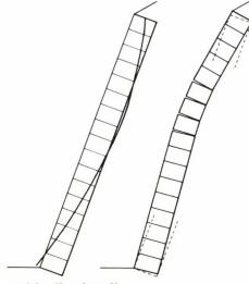
(a) Idealised wall (i) Thrust line (ii) Deflected shape *Fig. 5. Bulging failure modes on a rigid base*
