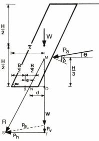
Fig. 3. Idealised section of upper H metres of wall
