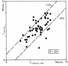
Fig. 5. Comparison of pile length
