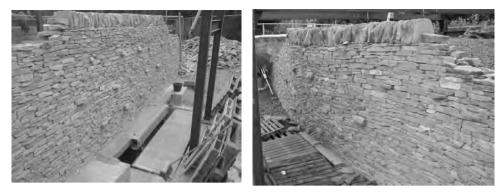
Figure 3: Test wall 1: a) post construction; b) prior to failure
